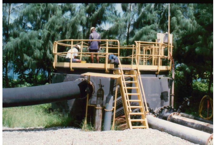
Tailings & Saltwater Mixing Tank at the Misima Mine, Papua New Guinea
